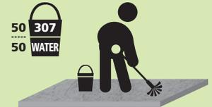
**Note:** for safety reasons, add **G-CLEAN 307** in water and not the opposite. **It is important to treat the concrete surface by 10m<sup>2</sup> (100 sq. ft.) sections.** If the product dries out OR is not rinsed properly, white salts deposits could appear on the surface. They are difficult to remove. Once applied on the surface, **it is important to flush the product with sufficient water.** Use a minimum of 20 litres of water per 10m<sup>2</sup> (100 sq. ft.) section.
