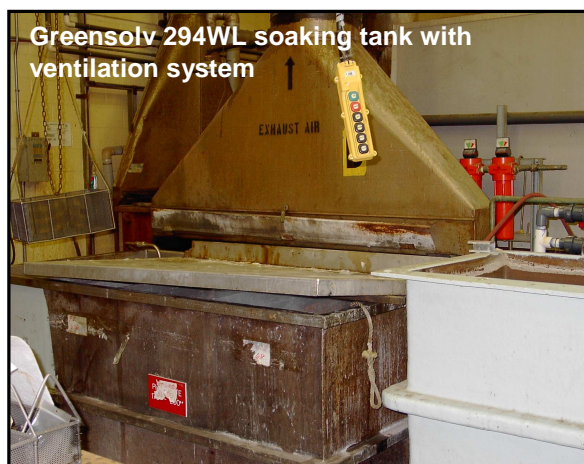
Magnesium parts stripped with Greensolv 294WL
